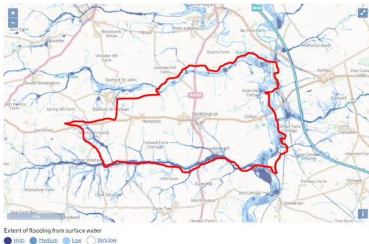
Figure B3.4 Surface water flood risk (approximate neighbourhood area shown in red)
